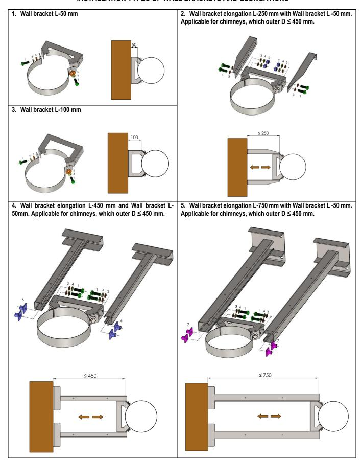
Fasteners: 1 -Bolt, 2 - Nut, 3 - Small washer, 4 - Spring washer, 5 - Big washer, 6 - Fastening plate 30x30, 7 - Fastening plate 40x40.
