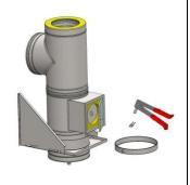
Pull connected components over the connecting flue pipe branch, mark points of attaching console to the wall. Attach the console with suspended wall support to the wall. The installer selects the method of attaching bearing elements to the wall.
