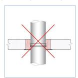
The joints of chimney sections in locations where it passes through a floor, roof or wall are not allowed
