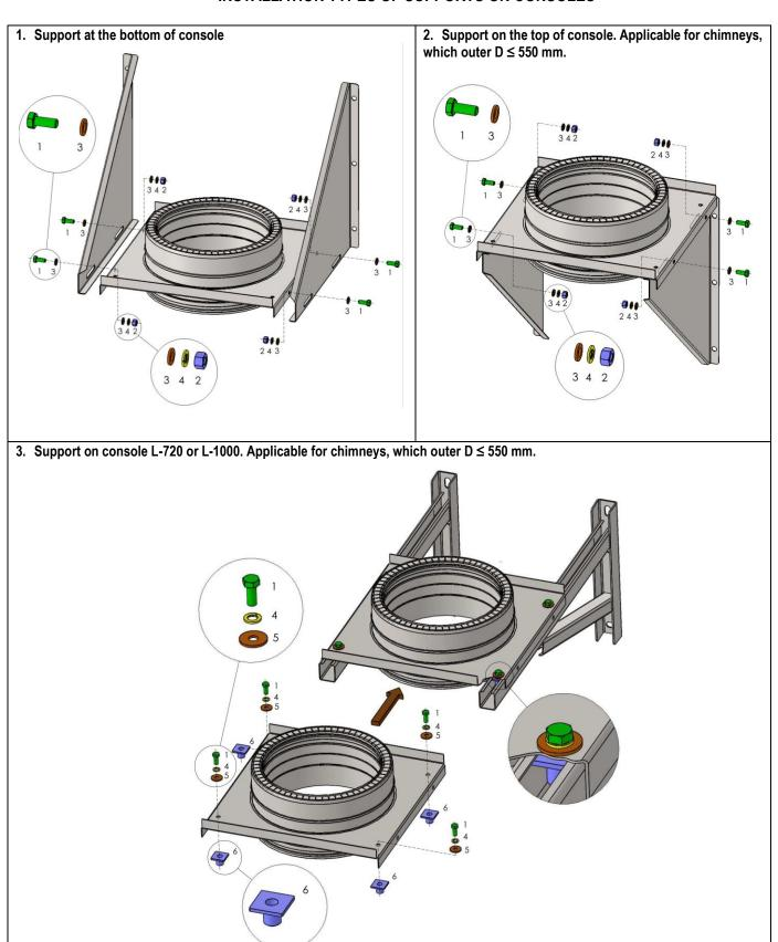
Fasteners: 1 -Bolt, 2 - Nut, 3 - Small washer, 4 - Spring washer, 5 - Big washer, 6 - Fastening plate 30x30.
